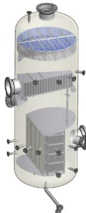
Isometric view of three-phase vertical coalescer/settler.
