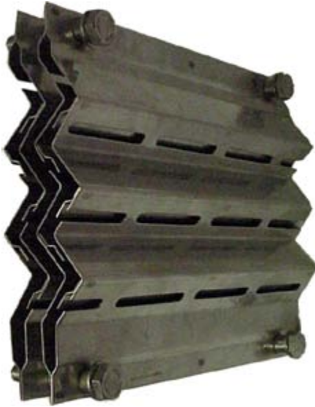
FLEXICHEVRON® style 350 high capacity mist eliminator for vertical gas flow.
